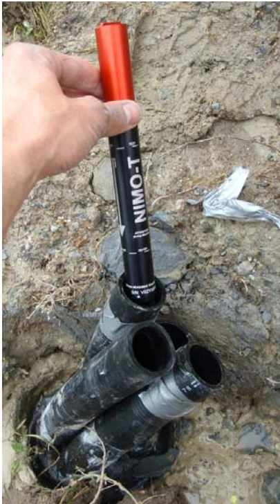
Fig. 2: Submersible temperature and pressure data logger and Fig. 3: Vertical temperature profiles in the fluid of the BHE at 3 different dates after the test
