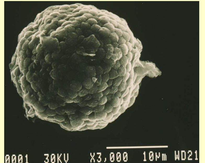
Initial Development of monosulfide rims (lower left) and even pyrite framboids (upper and lower right). Slide from previous papers.
