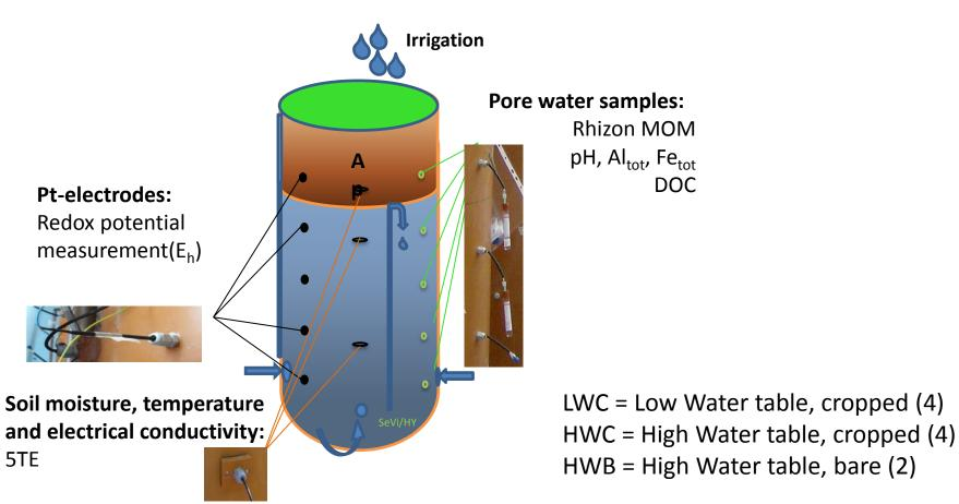
Eh, θ, T and EC were logged continuously.pH, Al, Fe and DOC in pore water were determined biweekly or monthly.
