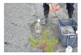
Fig. 3. Soil water sampling from an aggregate pile using a lysimeter. Photo: Timo Tarvainen, GTK
