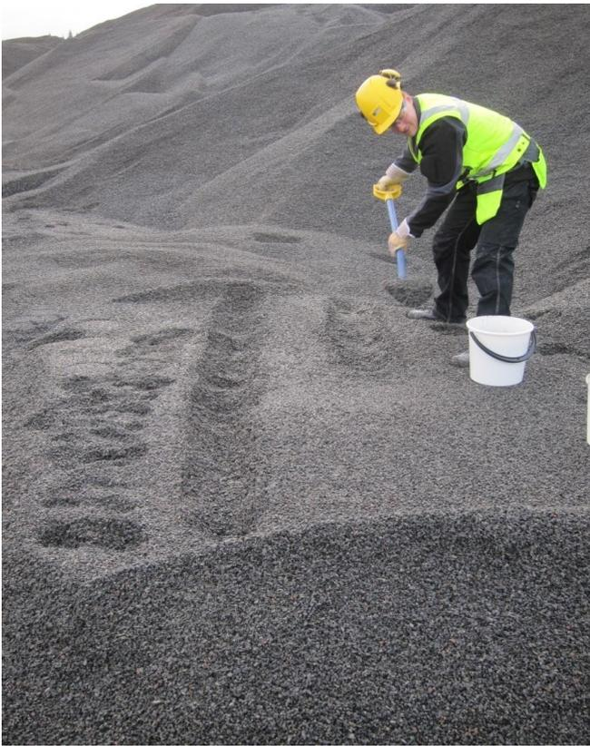
Fig. 6. Aggregate sampling for a leaching test.
