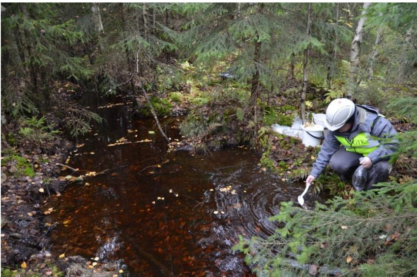
Fig. 9. Stream sediment sampling. Photo: Arto Pullinen GTK.
