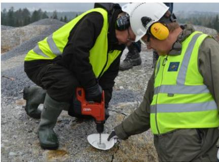
Fig. 1. Rock sampling using a hammer drill. Photo: Timo Tarvainen, GTK
