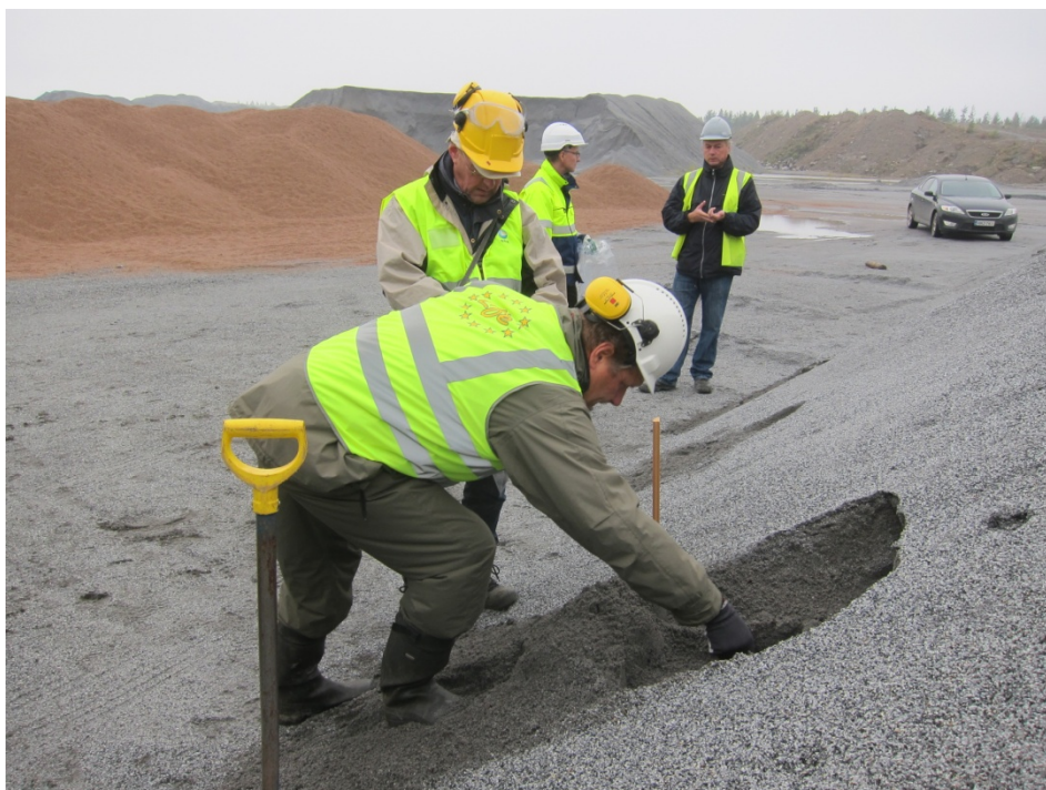
Fig. 7. The ASROCKS field work team is collecting a crushed rock aggregate product sample in the Nokia demonstration site during Action 2.
