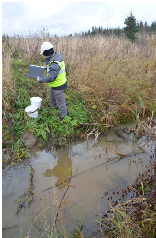
Fig. 5. Surface water sampling close to a demonstration site. Total and dissolved concentrations of arsenic and metals were determined for surface water and ground water samples.
