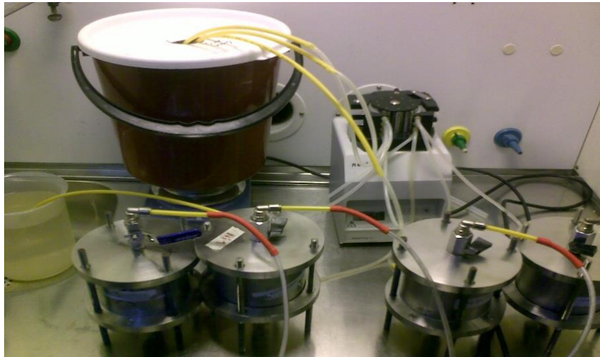
Figure 4. Laboratory scale adsorption columns (ECE, University of Oulu).
