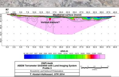
Detailed geophysical measurementselectrical resistivity tomography (ERT), induced polarization (IP), ground magnetic measurements, petrophysical measurements in the laboratory - are carried out by manual measurements in the field recordering the data and processing to produce interpretation maps to detect features on different depth scales. The geophysical interpretations are combined with the available geological knowledge to make a comprehensive model of the deposit.
