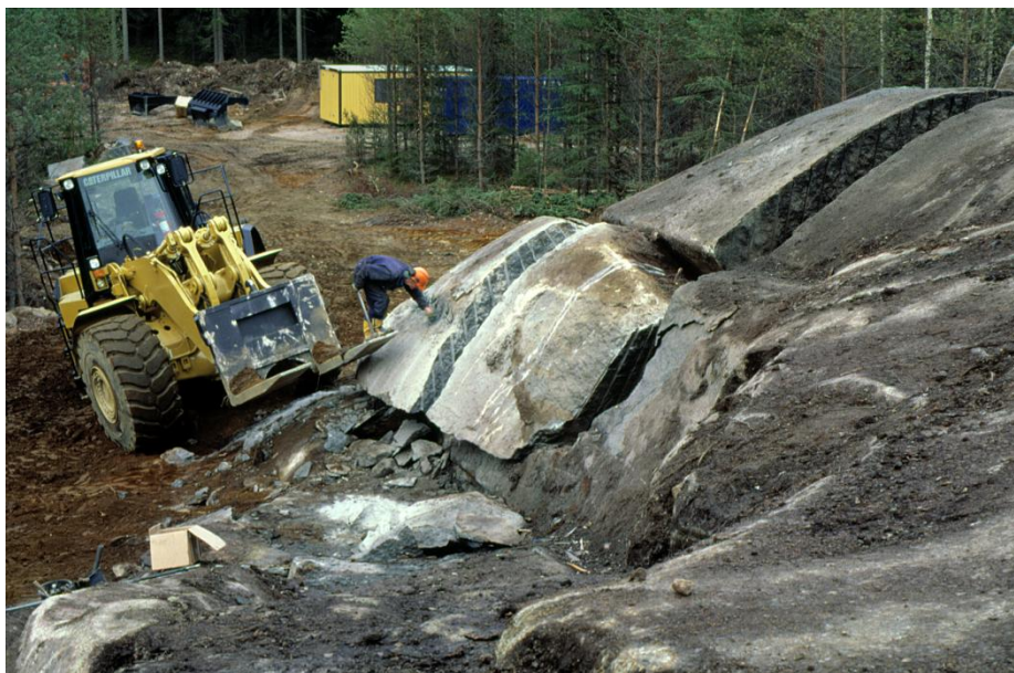
Fig. 30. The test quarrying tells the extraction properties of the rock. It also gives an estimation of the block size and yield of the deposit.
