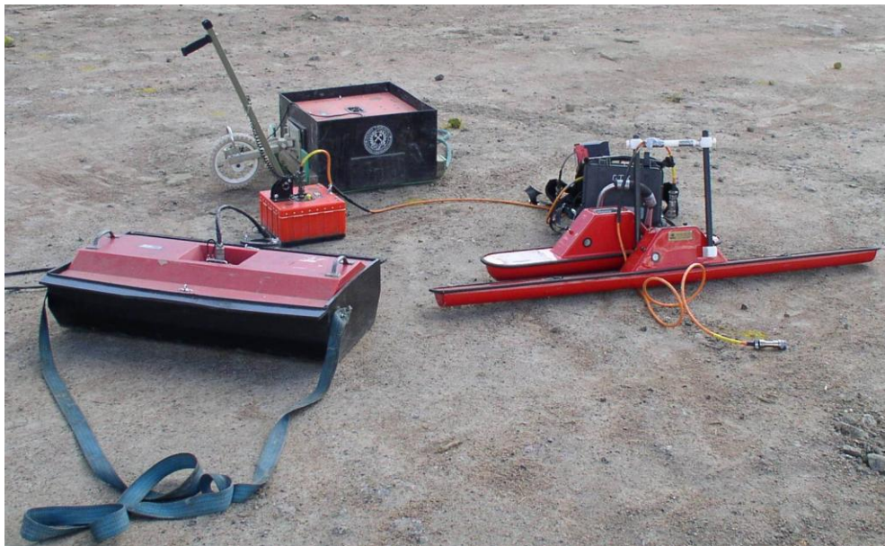
Fig. 22. Ground penetrating radar equipment used in exploration. The control unit (receiver) SIR-3000 and the antennae between 40 and 400 MHz.
