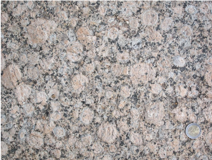
Fig. 20. A typical homogeneous rapakivi granite texture and colour observed from an outcrop. The stone texture is uniform and looks homogeneous.
