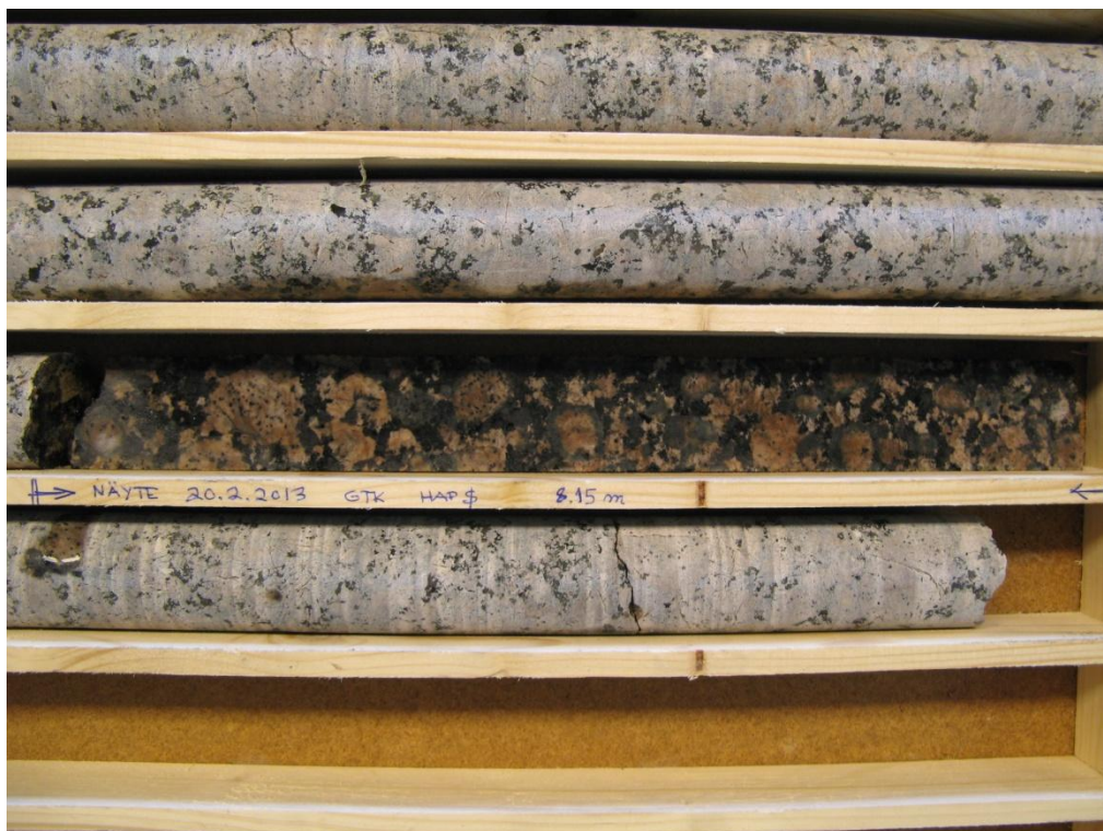
Fig. 29. Assessment of the stone texture, fractures and colour from the diamond drilling cores. In the middle, a drilling core has been split in two halves and the other side has been polished to observe better the colour and the texture.
