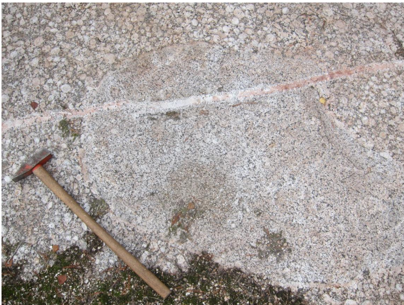
Fig. 21. Observation of the inconsistencies and defects on rapakivi granite. In this case there can be found a cross-cutting granitic vein and an inclusion of another rock type in the rapakivi granite.
