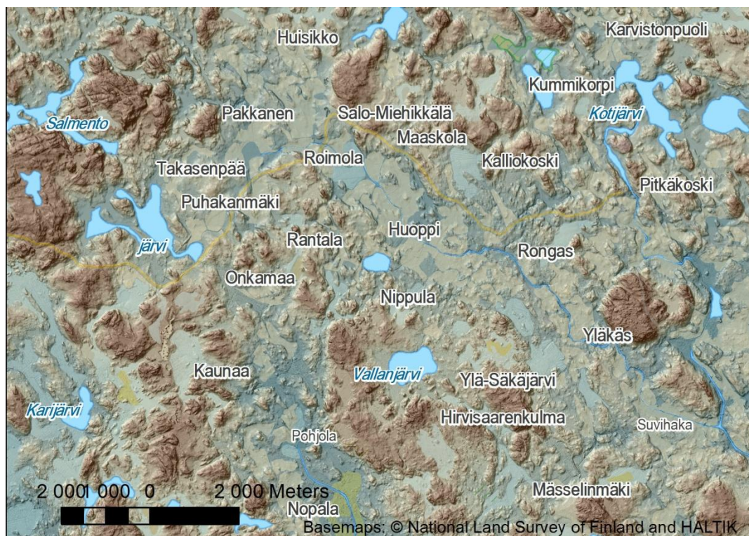
Fig. 10. An elevation map produced from airborne laser scanning elevation data.
