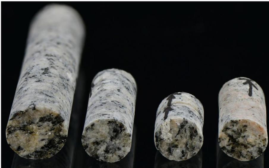
Figure 23. Back part of the drill cores collected, same as in figure 22, to evaluate the un-weathered surface of the material. (Photo by Jouko Ranua GTK)
