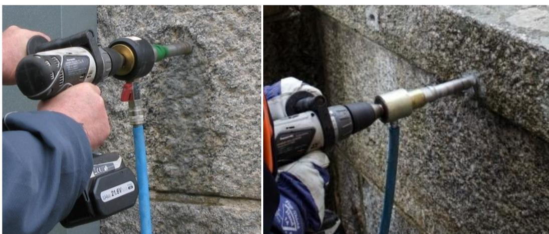
Figure 16 On the left the drill edge of 17 mm and on the right that of 20 mm. The drill is the same but the difference of diameter allowed collecting longer intact cores.
