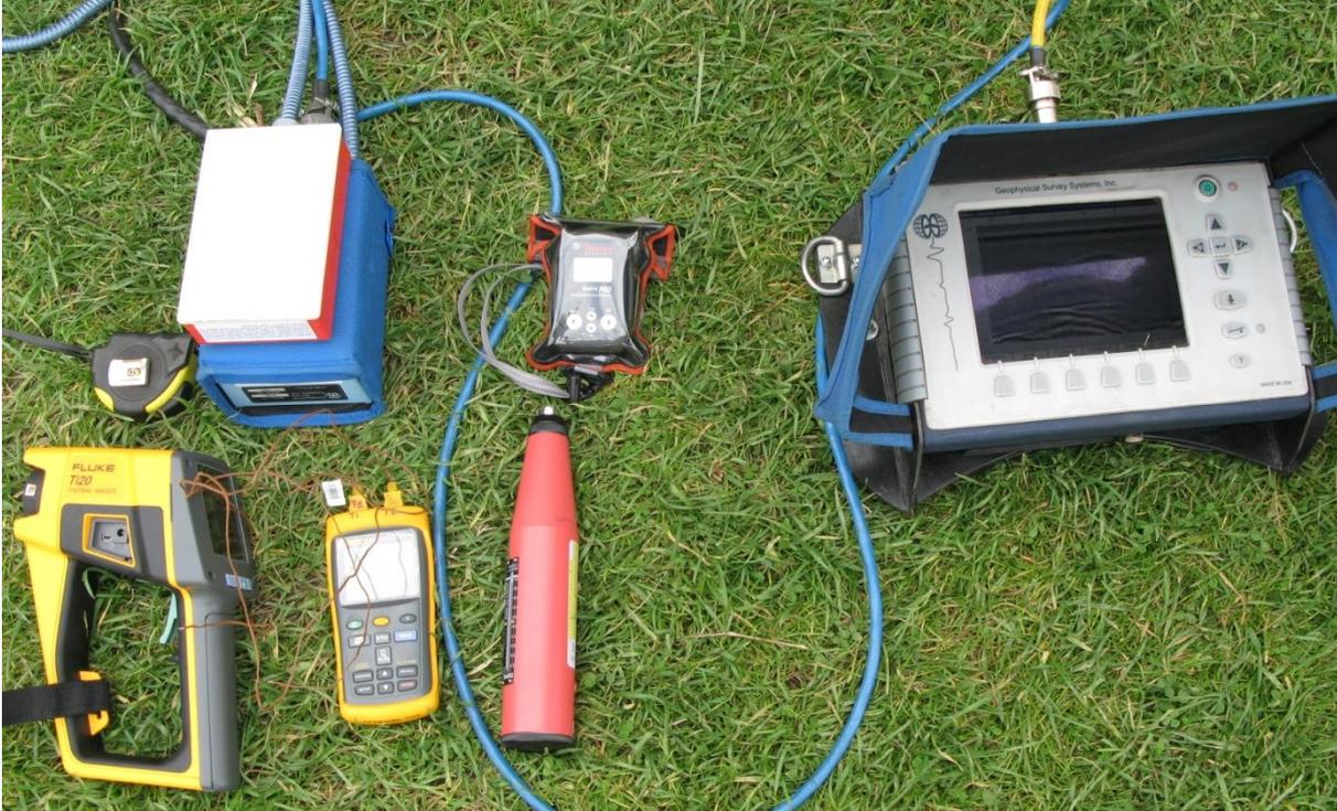
Figure 1 Thermal camera, thermometer, Schmidt hammer, ground penetrating radar, radiation pulse meter.
