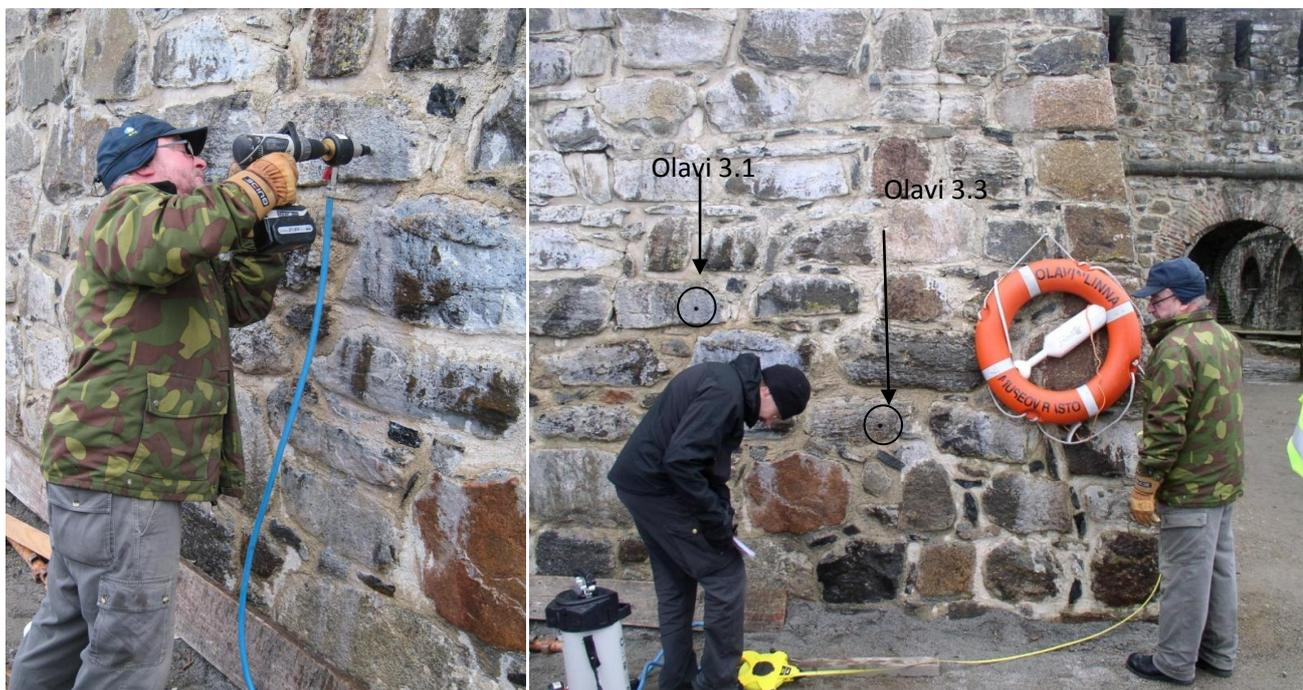
Figure 10. Sampling Olavi 3.1 (on the left), drill holes visible from the sampling of Olavi 3.1 and 3.3. on the bastions (on the right)
