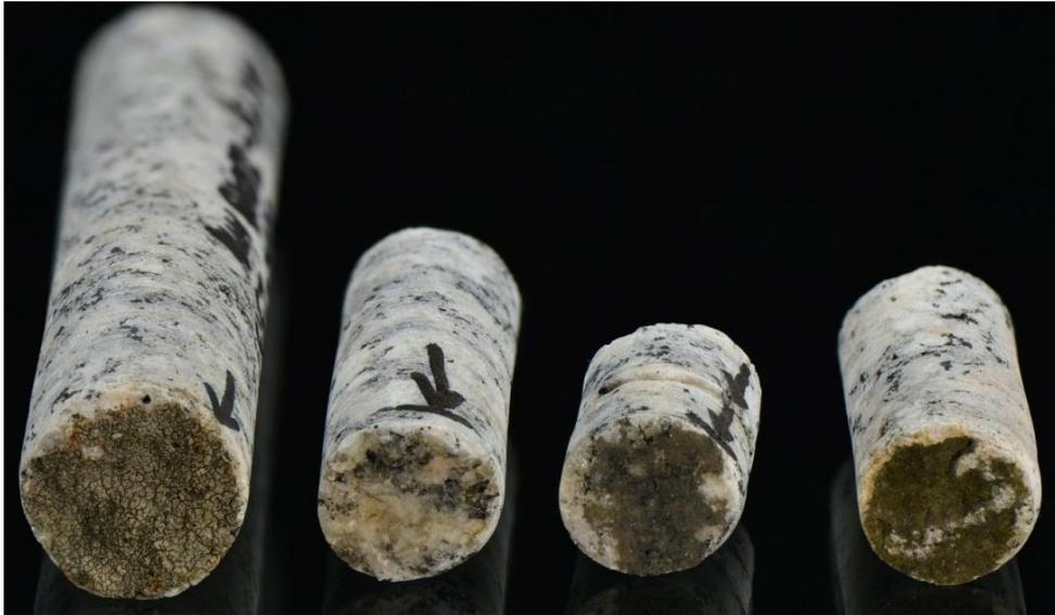
Figure 22. Weathered surface of the sampled collected from Niirala school, on the left the sample used for cutting the thin section. On the right three samples collected during 2012. (Photo by Jouko Ranua GTK)
