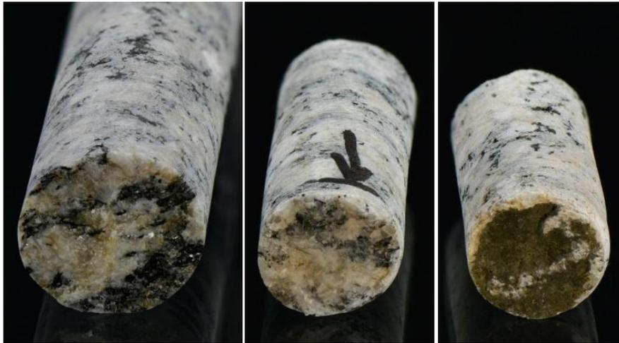
Figure 48. Samples used to evaluate the open porosity: HAPŞ -2012-25.3 (on the left), Niirala 1 (in the center) and Niirala 4 (on the right)
