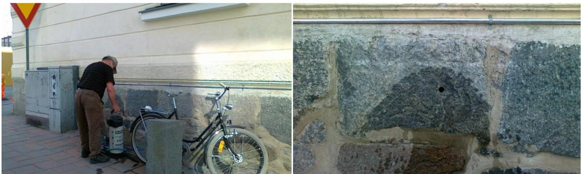
Figure 28 Sampling of "Lyseo 3" core taken from the basement dated 1874 on Hallikatu near the cross with Kauppakatu. The rock does not present deterioration problems (taken on 15.8.2012, photo Heikki Pirinen).
