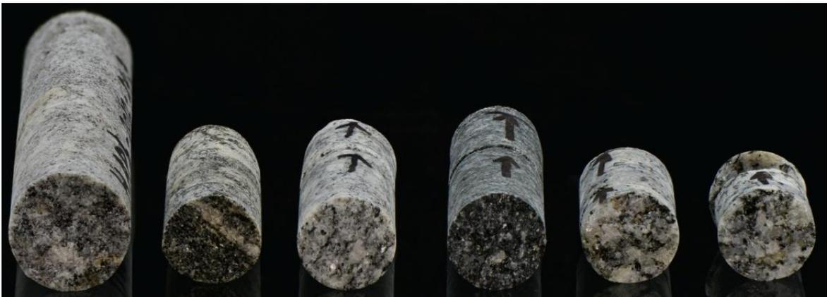
Figure 33 Back part of the drill cores collected, same as in figure 32, to evaluate the un-weathered surface of the material. (Photo by Jouko Ranua GTK)
