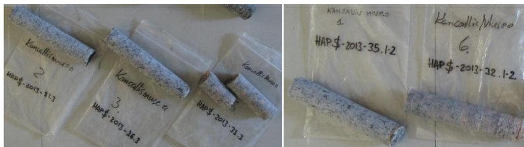
Figure 29. Normal photos of specimens from left to right HAP\$-2013-31,36,33 gone to petrographic analysis and HAP\$-2013-35,32 gone to chemical analysis. (photo:N.Luodes)
