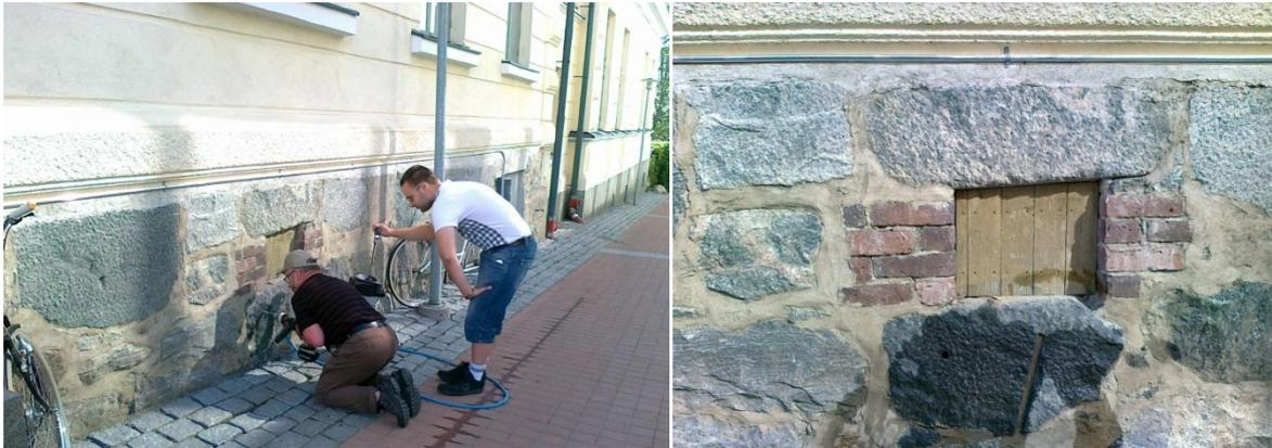
Figure 29 Sampling of "Lyseo 4" core taken from the basement dated 1874 on Hallikatu. The rock does not present deterioration problems (taken on 15.8.2012, photo Heikki Pirinen).
