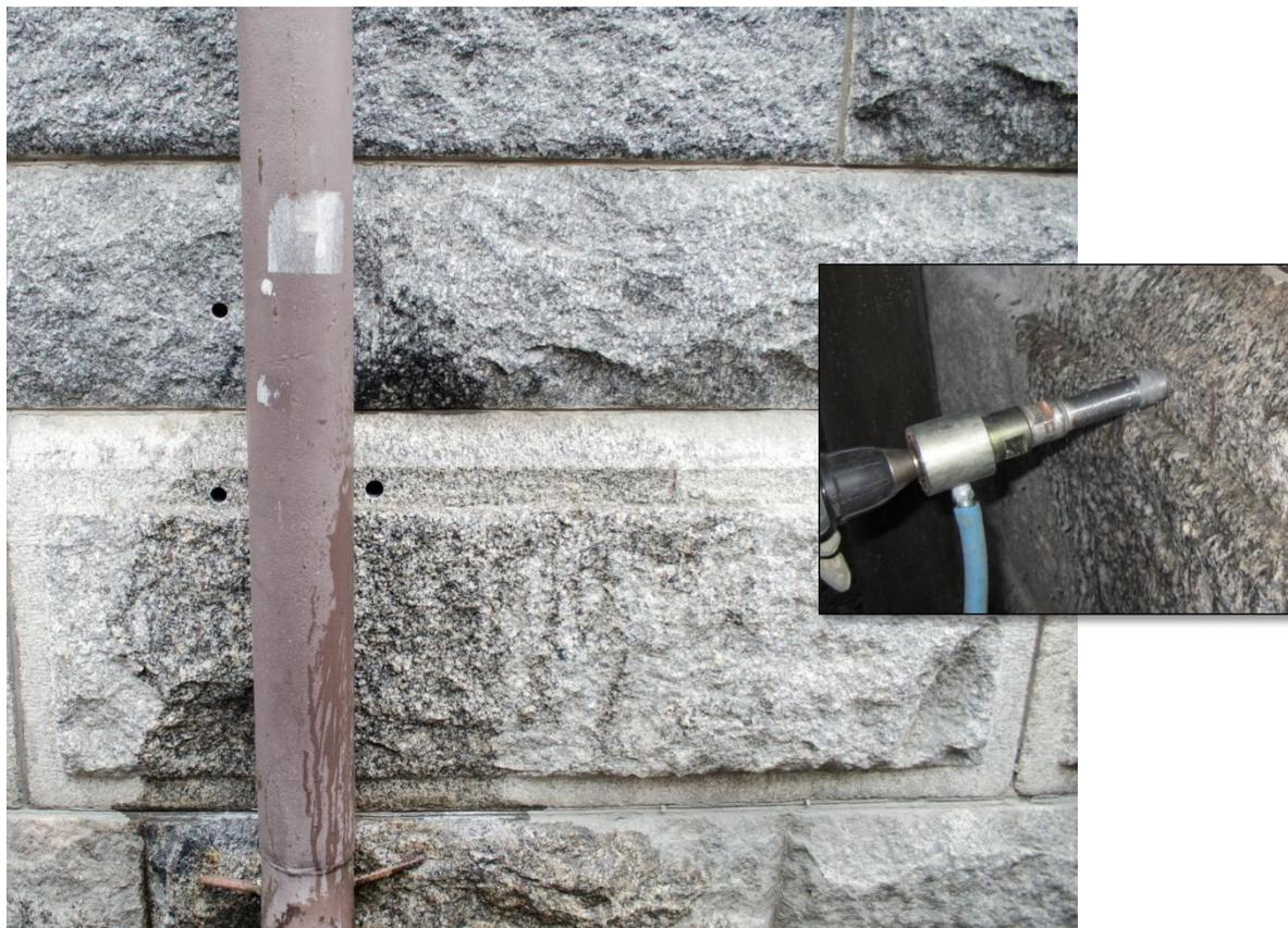
Figure 14 Sampling of HAPŞ-2012-22 (photo Joonas Toivanen)
