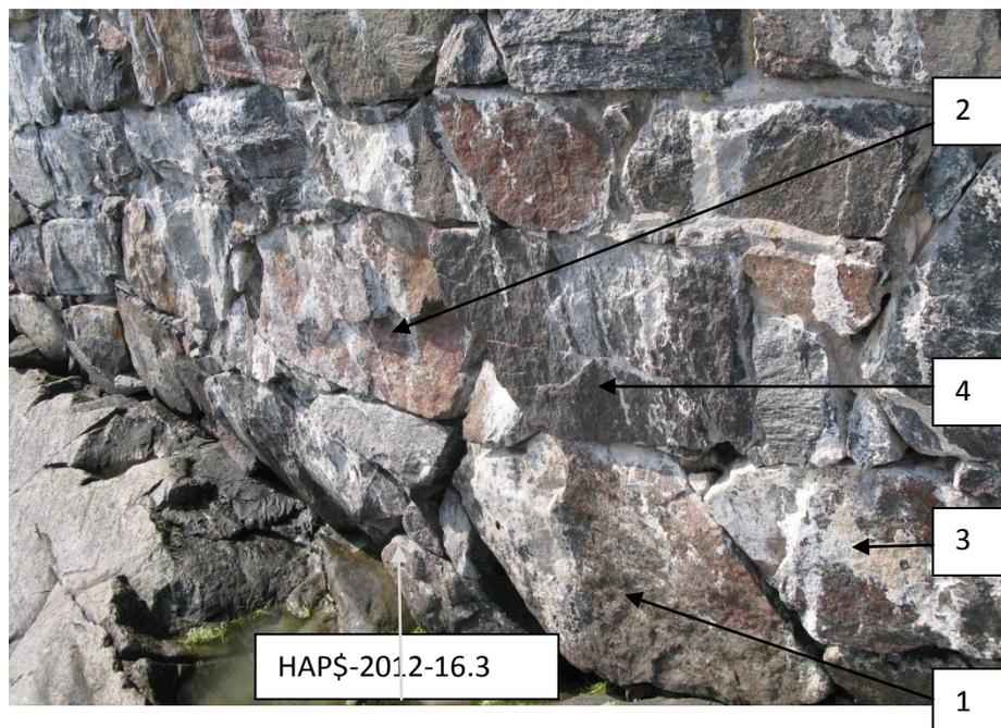
Figure 89 Schmidt hammer performed on the outer wall near the king’s gate
