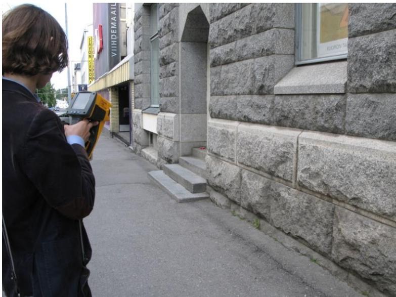
Figure 36. Collecting thermal images on site. (Photo: Nike Luodes)
