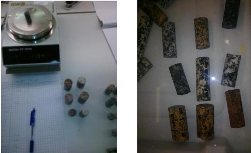
Figure 10. Testing of the drill cores for water absorption and density.
