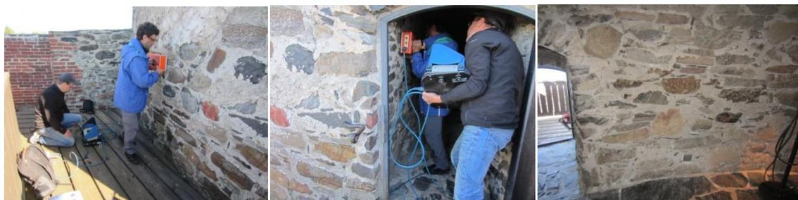
Figure 13 From left to right measurements performed over the outer wall, width of the wall, and inner wall of the Kello Torii
