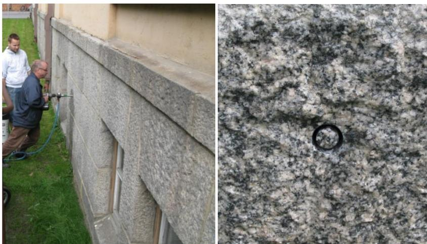
Figure 20 Drilling of sample Niiralan school 5 on the West basement façade on a stone not presenting weathering affects.
