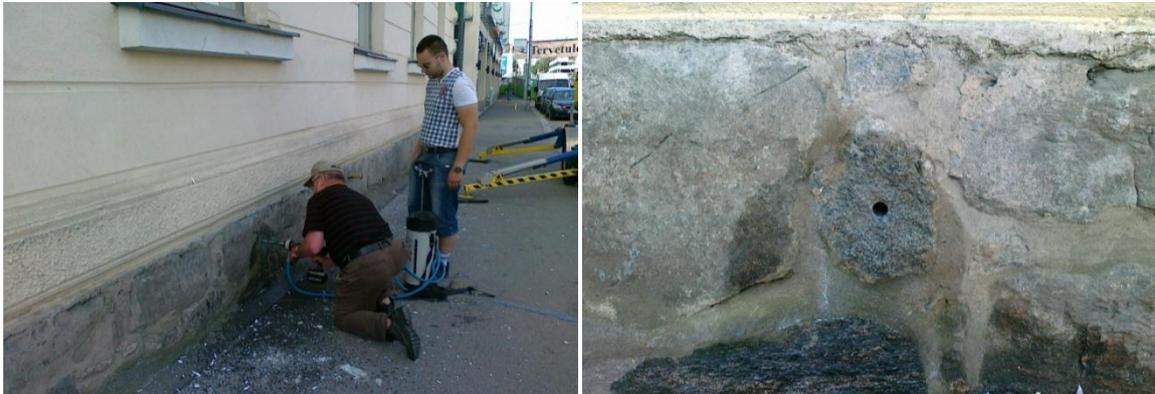
Figure 27 Sampling of "Lyseo 2" core taken from the old basement on the right of the main entrance door on Kauppakatu. The rock does not present deterioration problems (taken on 15.8.2012, photo Heikki Pirinen).
