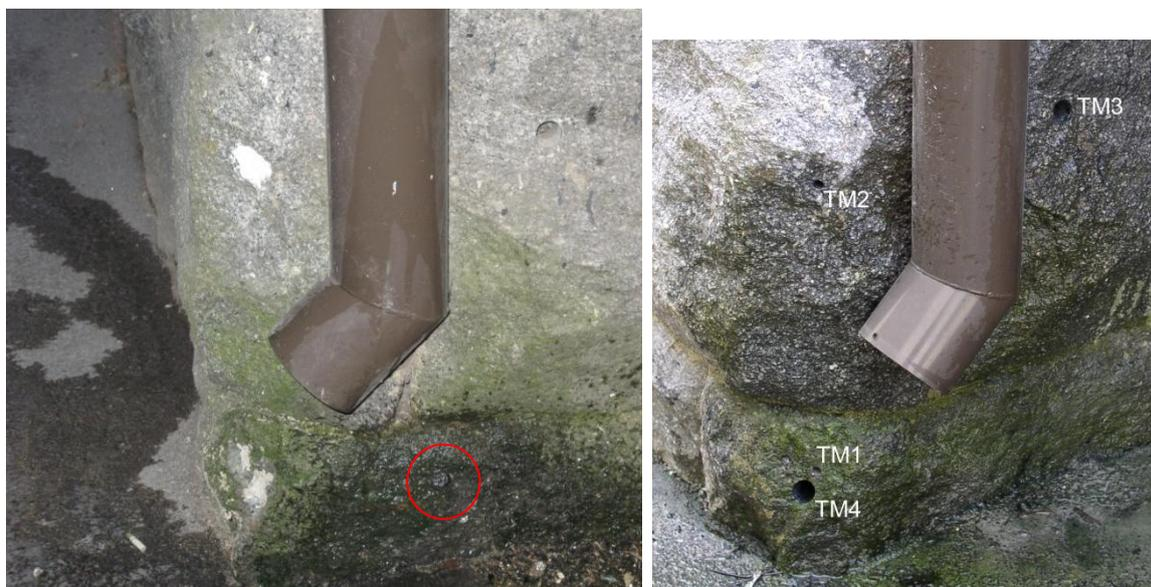
Figure 15 Sampling of HAPŞ-2012-23 (photo Joonas Toivanen, Heikki Pirinen). On the right are visible the first samples collected on 2012, with different drill edges.
