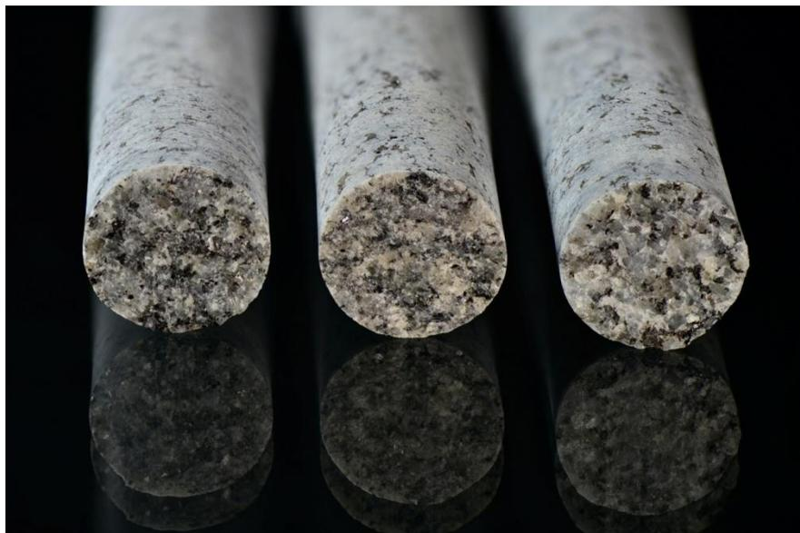
Figure 31 Back part of the drill cores, same as in figure 30, to evaluate the un-weathered surface of the material. (Photo by Jouko Ranua GTK) Samples from left to right: 31-35-36
