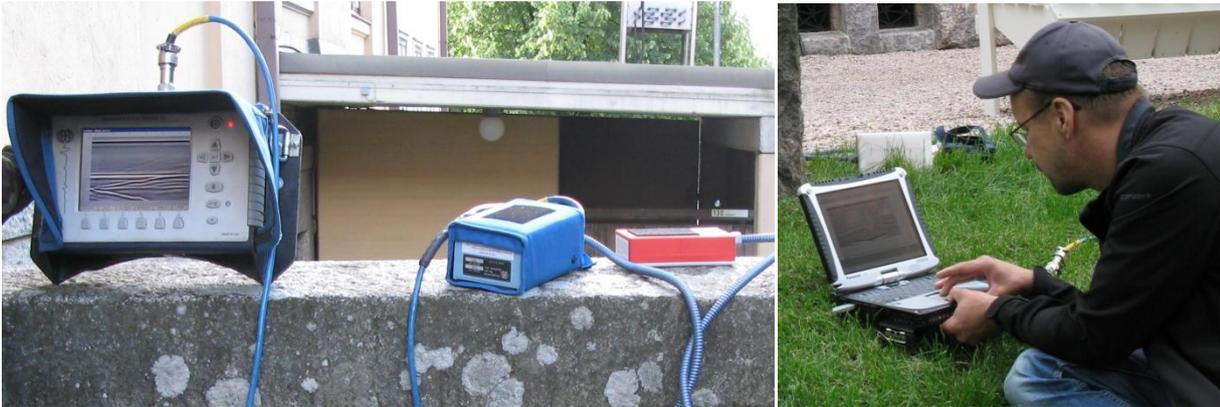
Figure 5. On the left SIR-3000 data acquisition unit with 1600MHz antennae, on the right evaluation of the results
