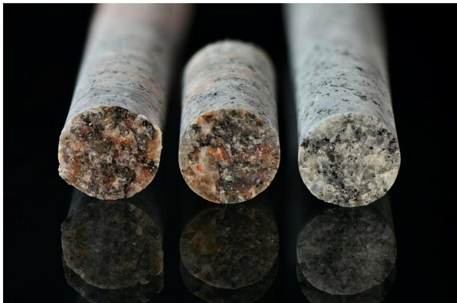
Figure 33 Back part of the drill cores, same as in figure 32, to evaluate the un-weathered surface of the material. (Photo by Jouko Ranua GTK) Samples from left to right: 32-33-34
