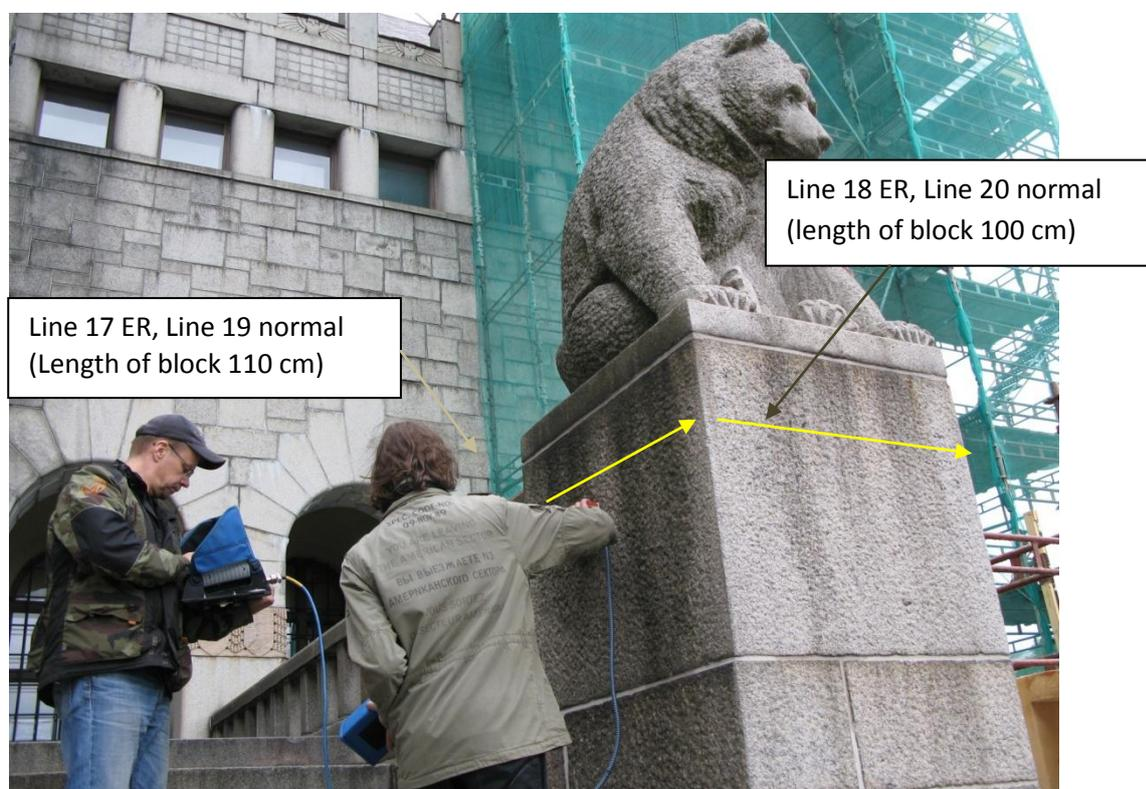
Figure 59. Measuring lines performed over the basement of the statue of the bear.
