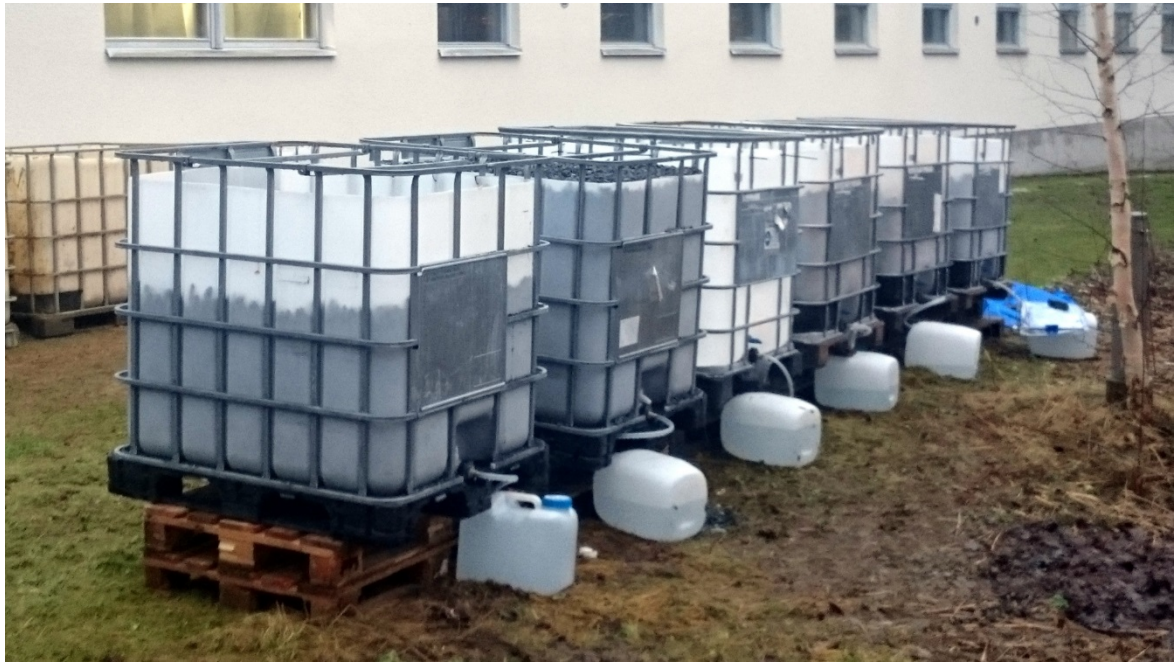
Fig. 1. Filled in lysimeters to study leaching behaviour of waste rocks in varying conditions. Photo © Teemu Karlsson, GTK.
