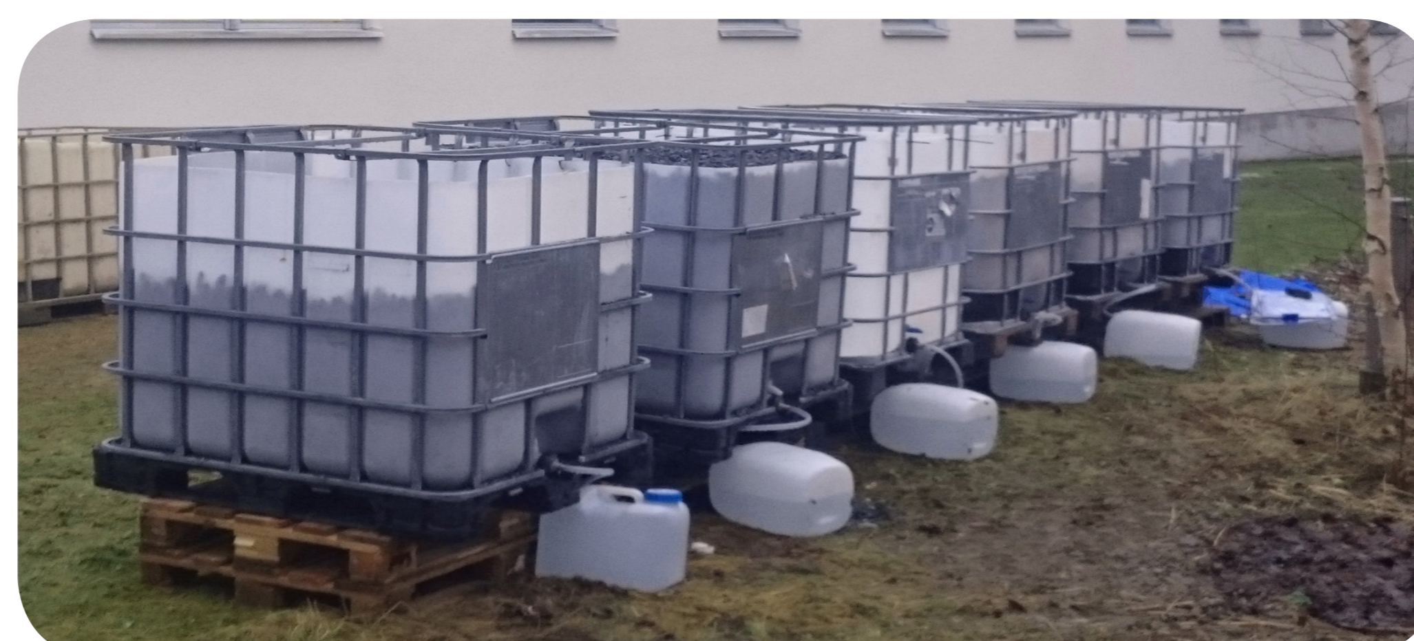
Figure 3. Filled in lysimeters to study leaching behaviour of waste rocks in varying conditions. Photo © T. Karlsson, GTK.
