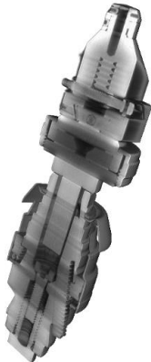
Drill chuck and goniometer as a split 3D tomographic visualization.
