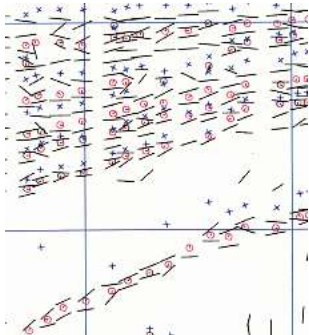
Fig. 12b. Directions of equal anomalies at maximum gradients (lines), total field maximums (circles) and minima (crosses) calculated from DC-3 data 1978. Flight lines are in NS-direction and 200 m apart from each other. The distance between co-ordinate lines is 2 km.
