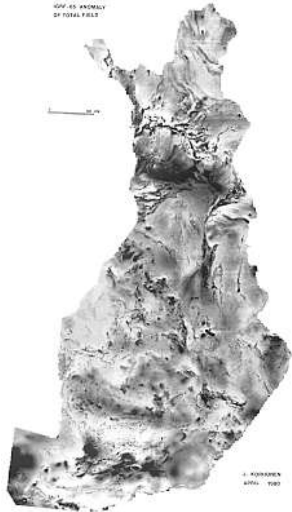
Fig 8. Magnetic High Altitude Survey (150 m) IGRF-65 anomalies in grey scales (50 nT interval, dark positive), original scale 1:2 000 000. The first grey tone map at the GTK in 1980, a by product of printing the Magnetic Anomaly Map of Finland (Korhonen 1980)
