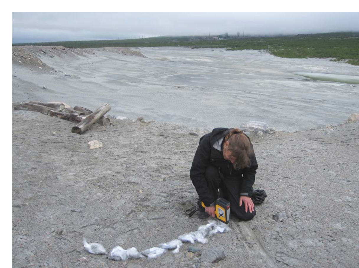
XRF measurements in the tailings of the Umbozero Mine, Russia.
