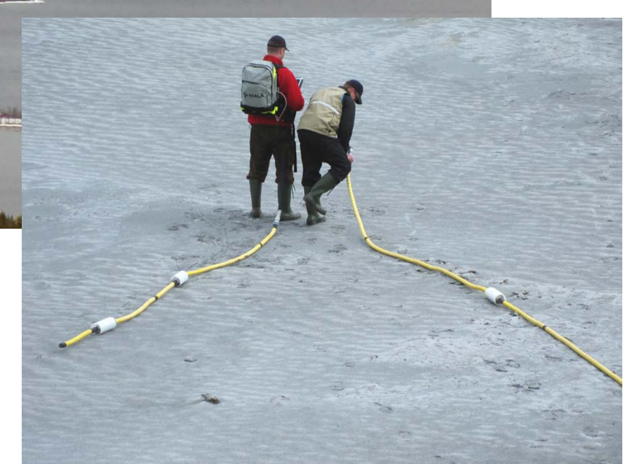
Field studies by GPR in the tailings of the Umbozero Mine, Russia.
