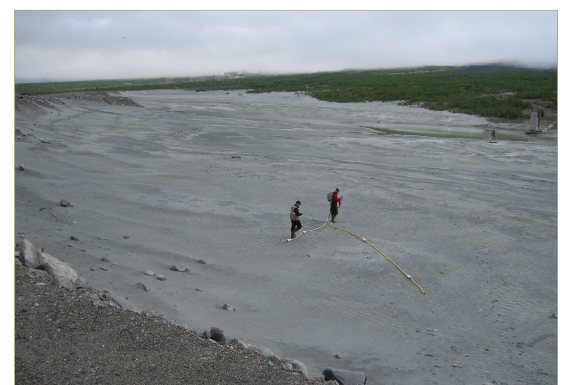
Field studies by GPR in the tailings of the Umbozero Mine, Russia.
