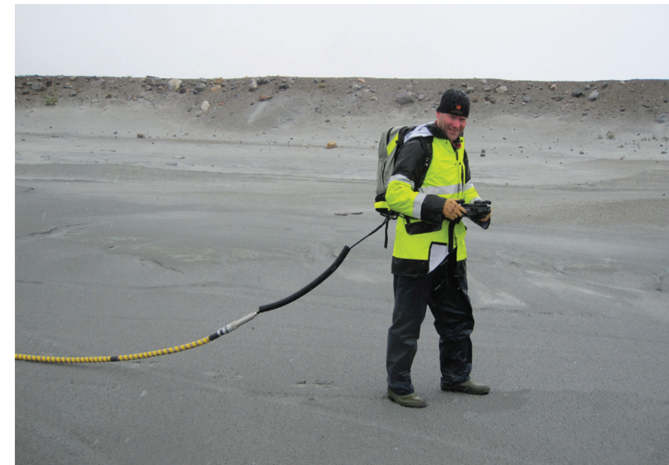
GPR measurements at the tailings, Umbozero.
