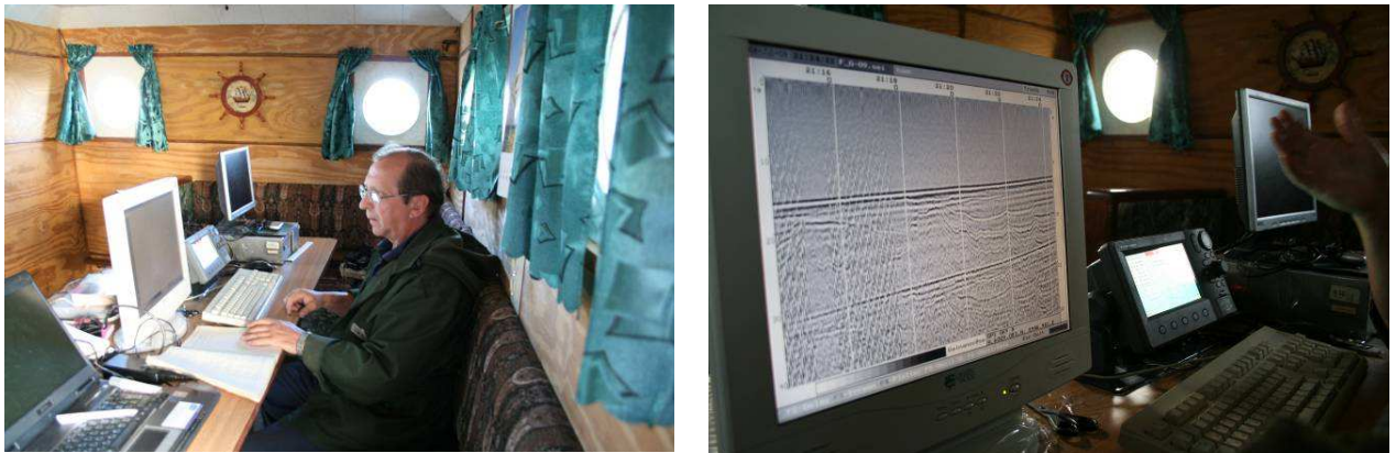
Figure 5. Work with geo-acoustic complex GEONT-HRP ("Spektr-Geophysika" Ltd.).
