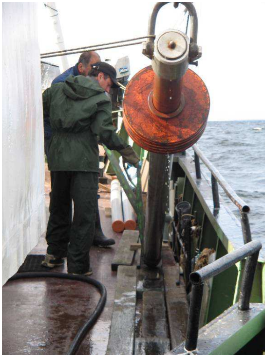
Figure 7. Work with gravity corer on board r/v Ladoga.
