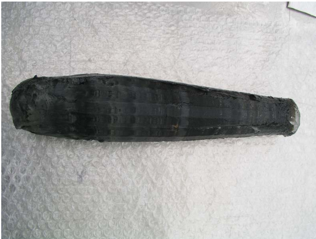
Figure 6. Frozen surface sediment sample taken using mini ice finger. Photo: Aarno Kotilainen, GTK.
