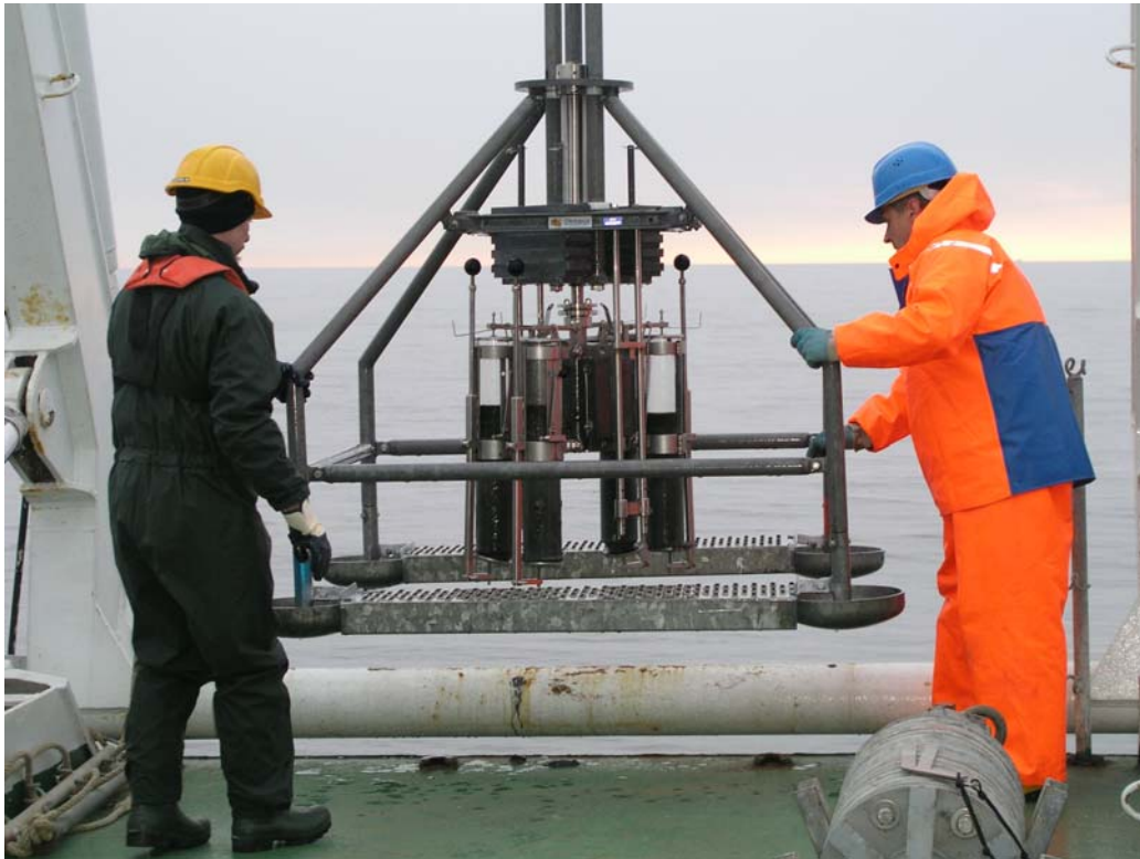
Figure 4. Multicorer in use onboard RV Aranda. Photo: Aarno Kotilainen, GTK.
