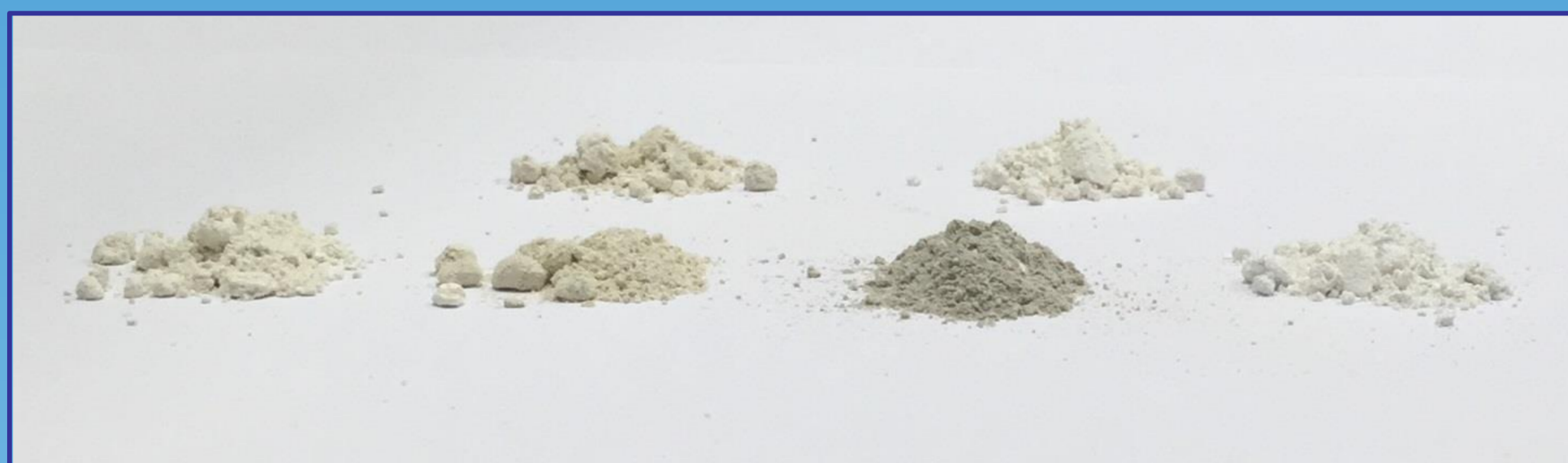
Fig. 1 From left to right in the foreground by-products A-D, in the background quicklime and hydrated lime.
