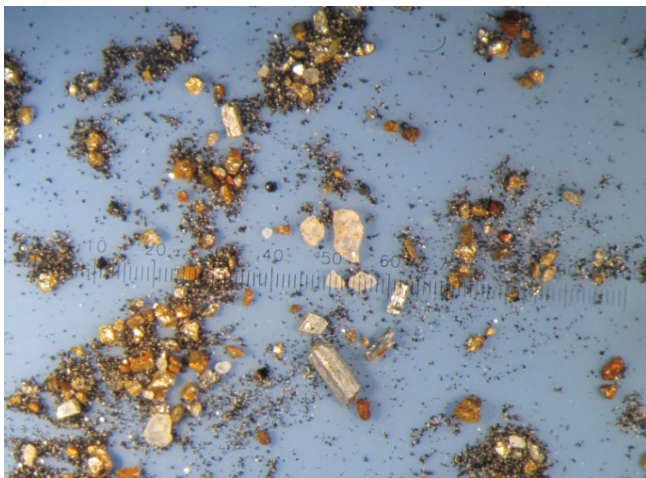
Figure 1. Arsenopyrite and scheelite found in glacial drift, one small gap in scale equals 0.1 mm.
