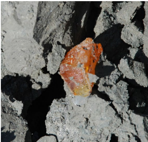
Figure 4. Glauconite sand with amber. Prospecting for amber, Górka Lubartowska Deposit, Natural size.
