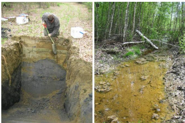
Figure 4. Sampling of tailings and surface waters in the vicinity of the closed Haveri Cu-Au mine. The upper part of the tailings layer is clearly oxidized. The surface waters contain significant amounts of heavy metals.
