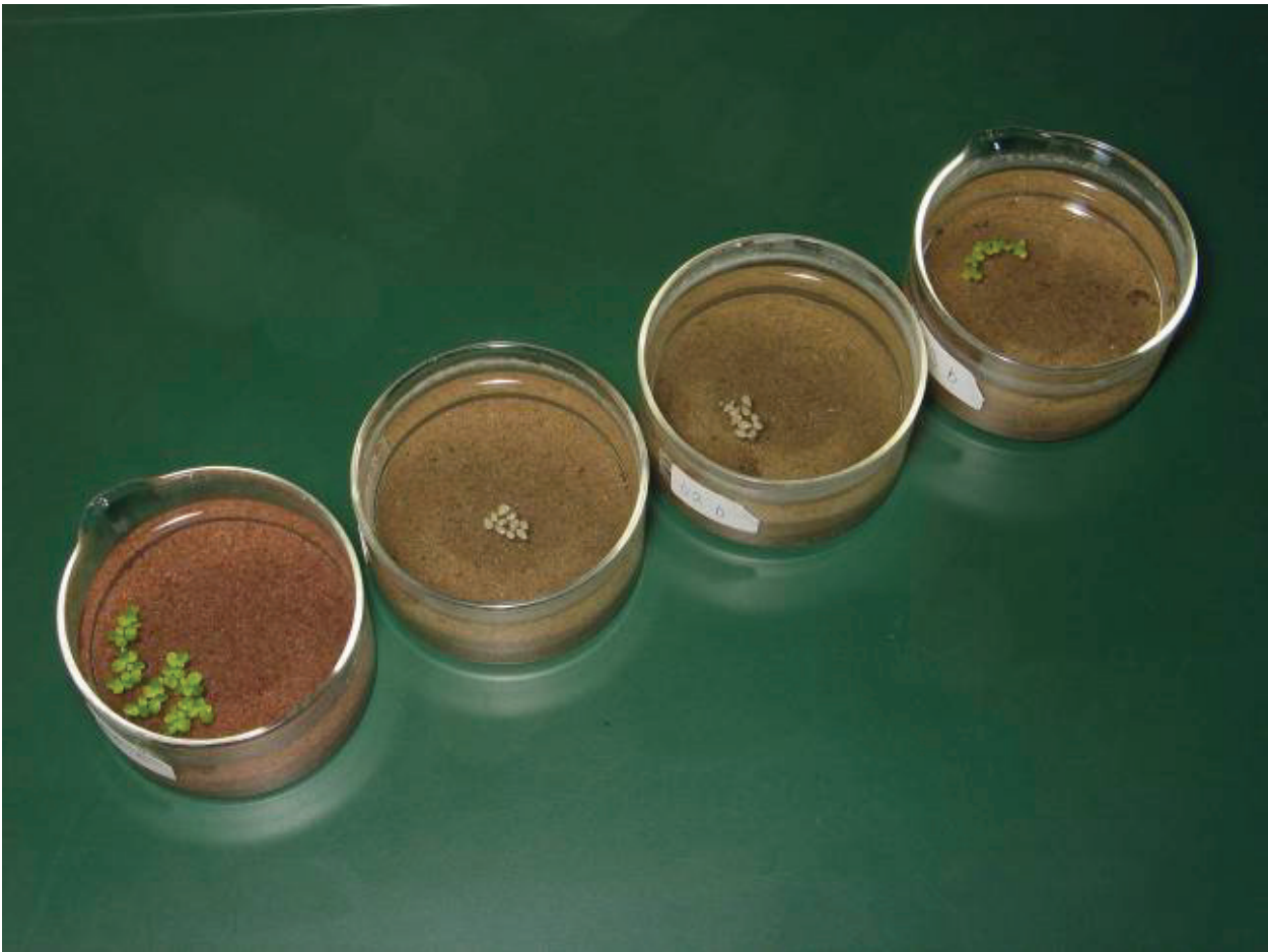
Figure 5. The final stage of the growth inhibition test using Lemna minor , tests with soil samples from the CCA plant site and control soil (on the left). The test plants were grown one week in a vessel containing 50 g of soil sample and 100 ml nutrient solution. At the start of the test, there were 10 leaves in each vessel.
